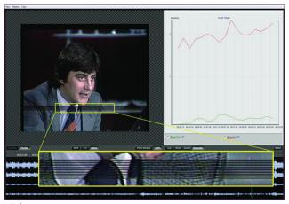
Figure 6: Burned-in defect.
