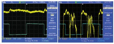
Figure 2: Normal RF envelope vs. Drop-out pattern
