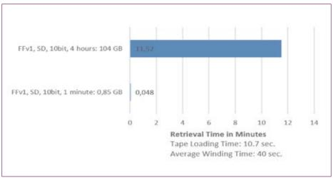
**Figure 8.** Comparison of retrieval times on LTO 7.
