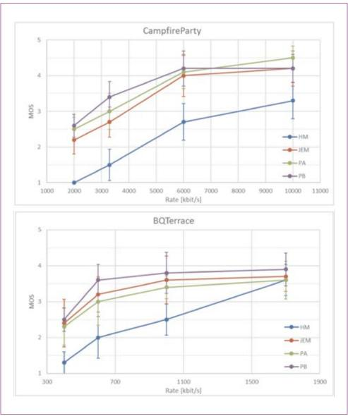
**Figure 10.** Subjective evaluation of two video clips, each coded using four codecs at a range of bitrates, from Baroncini, et al., 2017.
