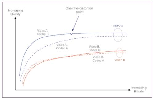
Figure 9. Rate-distortion curves: two clips and two codecs.
