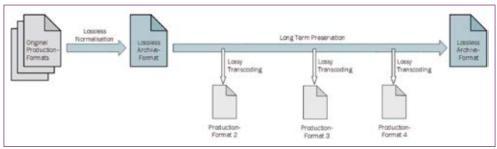
Figure 6. Transcoding history without generation loss.
