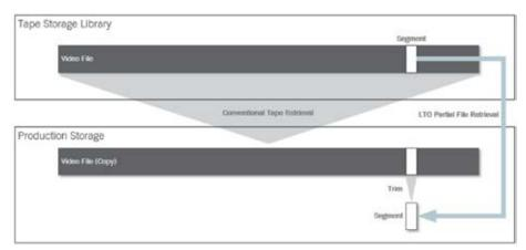
Figure 7. Schematic partial file retrieval.
