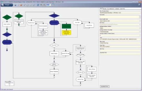
**Figure 12.** Workflow (NOA mediARC) describes the tasks in the background fulfilling export from a lossless FFVI archival format to AVCIntra 100 incl. 3rd party video QC engine.
