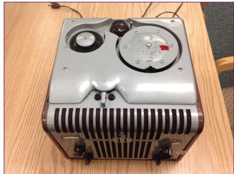
Figure 1: Webster-Chicago Electronic Memory Wire Recorder, Model 81-1.
