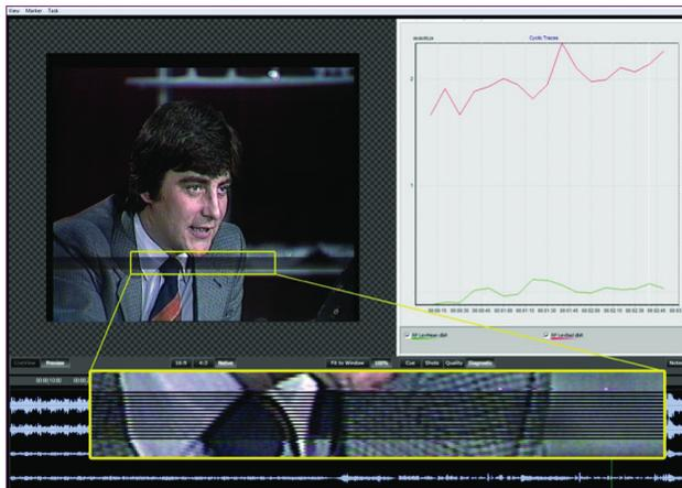
Figure 6: Burned-in defect.
